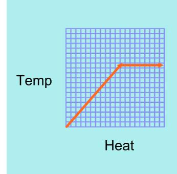
the flat part shows a change in state. All energy is being used to boil the water.
